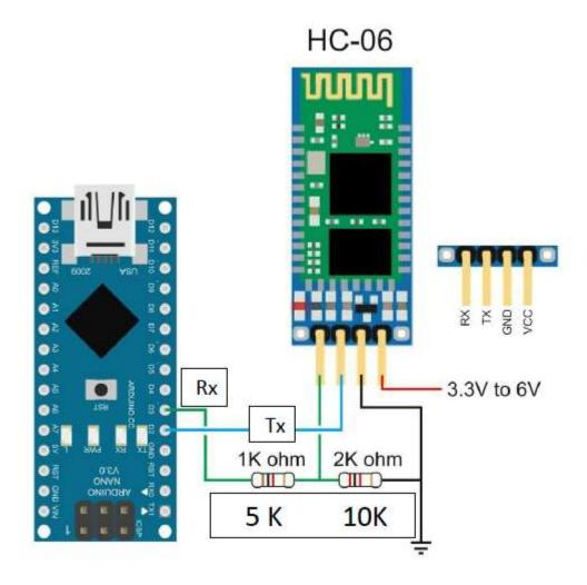
The drawing represents an Arduino NANO, instead of an UNO, but the schematic just wants to describe the resistors' partition, so to preserve the HC06 Rx pin.
